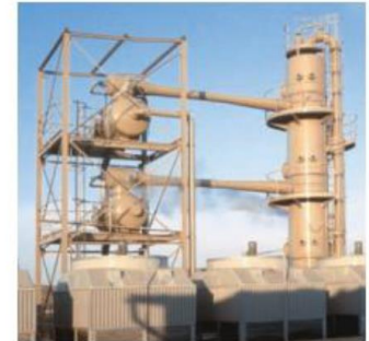
Fig. 9: 3-stage steam jet cooling plant of bridge design, cooling 194 m 3 /hr of water from 28 to 15 °C. Chilling capacity: 2 900 kW
